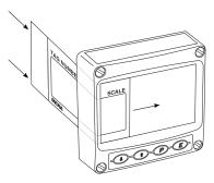
Fig 4 Inserting scale card into the instrument assembly.
