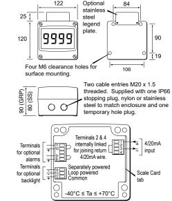
Fig 2 Dimensions and terminal connections
