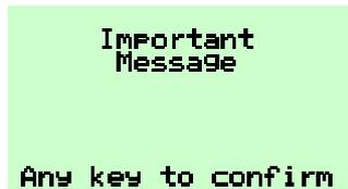
Wait for an operator response by checking the KEY\_STATUS parameter in the transducer block.
