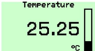
Standard Screen 6 is being used to display an  $IN_1$  value in degrees Celcius.
