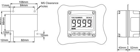
INSTRUMENT PANEL THICKNESS: 2 to 5mm
