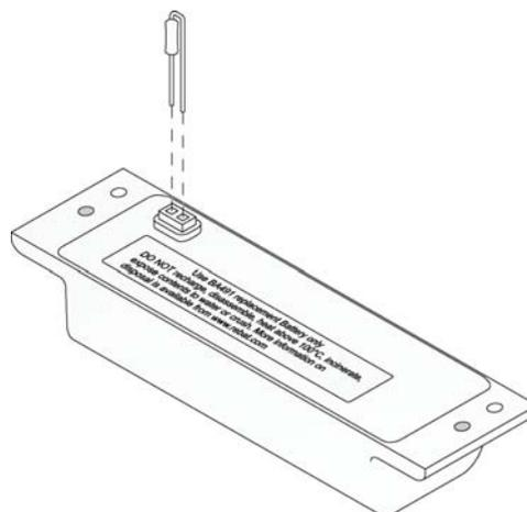
Fig 1 Condition BA491 battery by plugging 27Ω resistor into output terminals for about 30 seconds.
