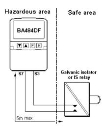
Fig 3 External push-button switch in safe area
