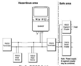
Fig 2 FISCO fieldbus system
