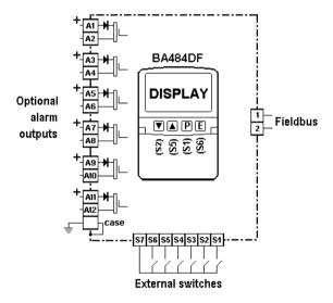
Fig 1 Simplified block diagram of BA484DF-F
