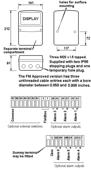
Fig 6 Dimensions and terminal connections
