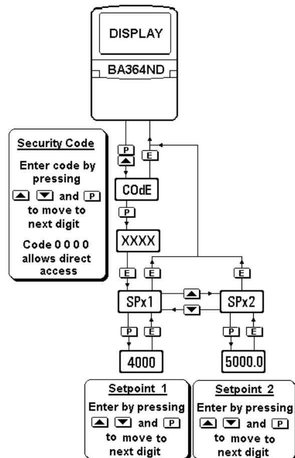
Fig 4.4 Setpoint adjustment from the display mode
