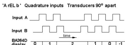
To achieve reliable counting from a quadrature encoder the two input signals do not require equal marks and spaces, but input A must not change state for 100µs before or after input B as shown in timing diagram below.
