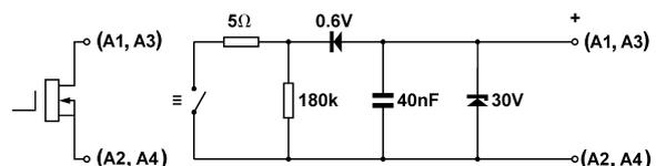
Fig 1.5 Equivalent circuit of each control output
