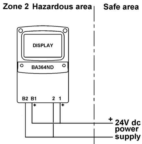
Fig 1.8 Connections for backlight
