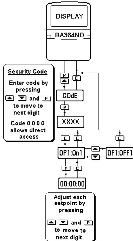
Fig 5.3 Setpoint adjustment from the clock display mode
