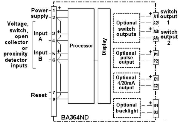
Fig 1.1 Simplified block diagram of BA364ND
