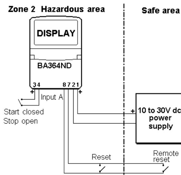
Fig 3.4 Starting & stopping timer with one input
