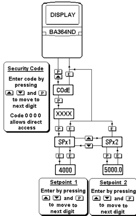
Fig 2.4 Setpoint adjustment from the display mode
