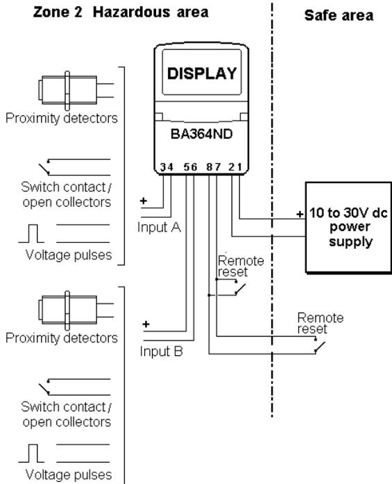
Fig 2.1 Typical counter installation
