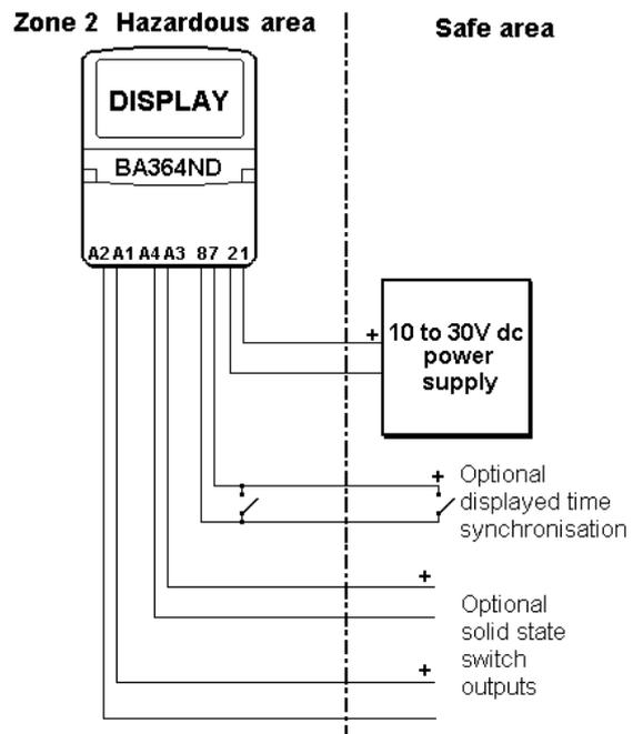
Fig 5.1 Clock installation
