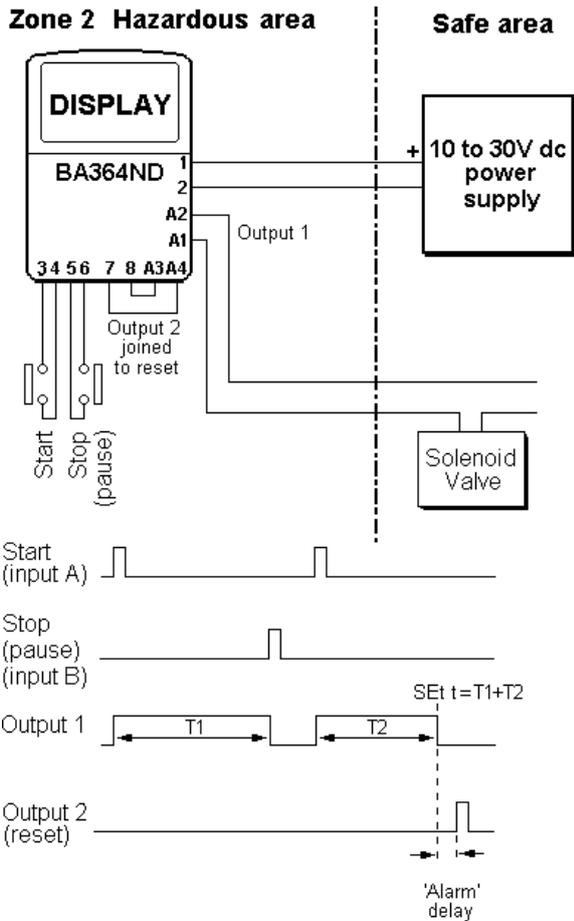
**Note:** When the elapsed time (T1+T2) equals the set time SEt t, an internal stop signal is automatically generated which stops the timer and opens control output 1.
