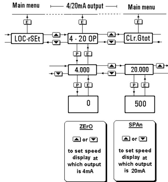
Fig 4.5 4/20mA output programme structure
