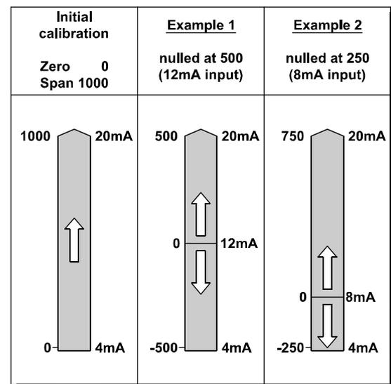
Fig 8 Effect of nulling at two different inputs
