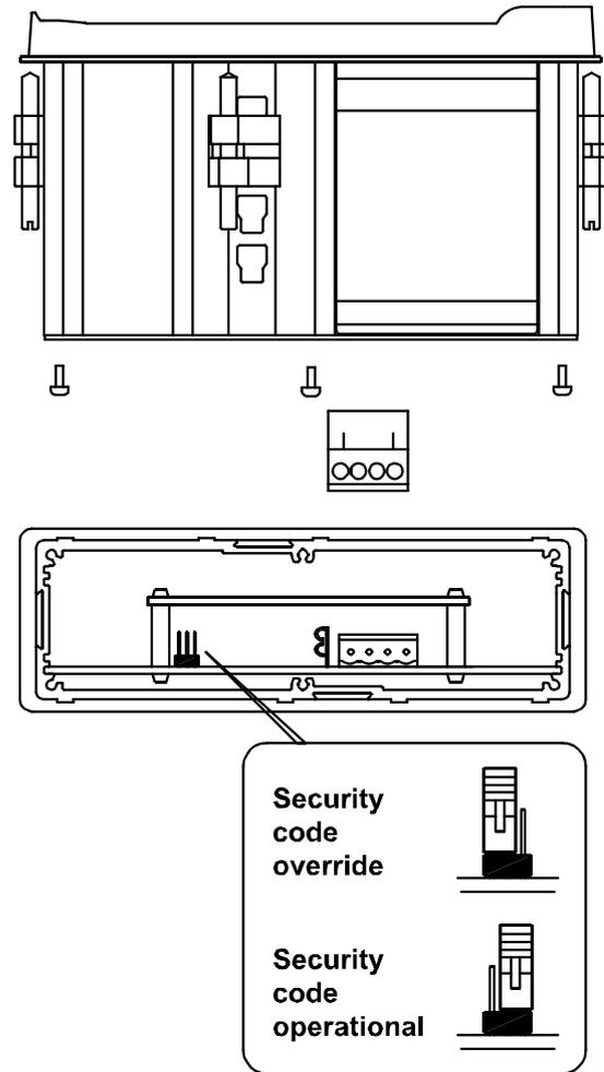
Fig 9 Location of security code override link
