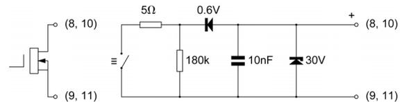
Fig 12 Equivalent circuit of each alarm output
