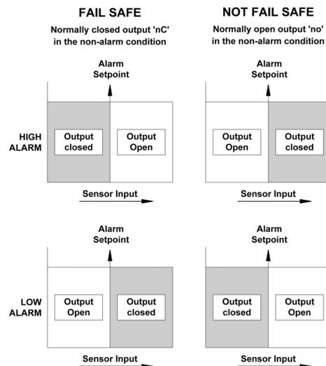
Fig 10 Alarm outputs
