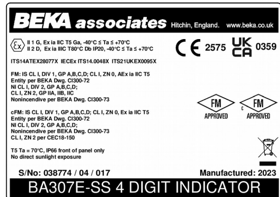
BA307E-SS intrinsic safety certification label
