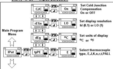
This function allows the setting of the input type, the units of display ( $^{\circ}$ C or  $^{\circ}$ F), the display resolution and the cold junction compensation.
