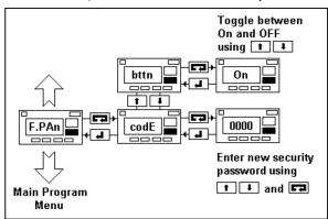
parameter is set to "off" then the pushbuttons will be disabled (to re-enable see section 8.7). The security password set in "CodE" is the password required to gain access to the Programming Mode. If password controlled access is not needed, the code should be set to "0000" (four zeroes).
