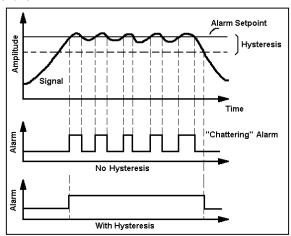
**8.6.2) "EnbL" – Enable**. This parameter enables an alarm to be easily switched on or off without having to change all the other alarm parameters. **NOTE:** If the alarms are not enabled, the alarm relays will stay in the position determined by the "nE" (normally energized) parameter.
