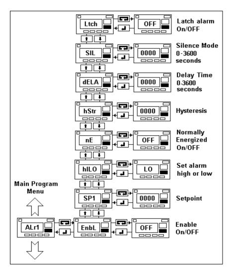
**8.6.6) "dELA" - Delay**. This function can be programmed to delay alarm activation by up to 3600 seconds. If set to "0000" then there is no delay in the alarm.
