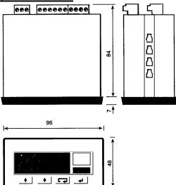
Recommended panel cut-out: (dimensions in mm) DIN43 700. 92.0+0.8/-0.0 x 45+0.6/-0.0
