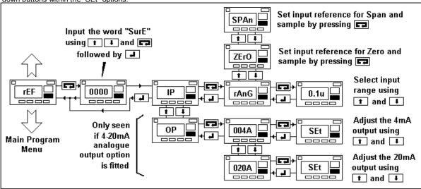
Please note to ensure maximum accuracy, whenever the input signal range of the indicator is changed as outlined in section 8.5.7, (for example, change the input from 0-10V to 4-20mA), the display should also be re-calibrated as outlined in section 8.5.6.
