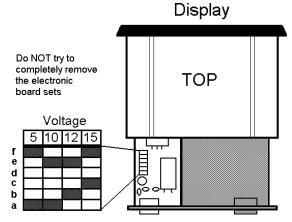
NOTE: The electronic circuit board sets are not designed to be completely removed from the case !! Position the links in the appropriate places (e.g. 12Vdc supply requires links to be in position b and e) and carefully re-assemble. The transducer supply is short circuit protected.
