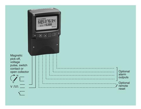
The BA544D is a battery powered rate totaliser with separate rate and total displays. An accumulated grand total may also be displayed. The instrument will count switch contact closures, voltage pulses and the low level output from magnetic pick-offs.
