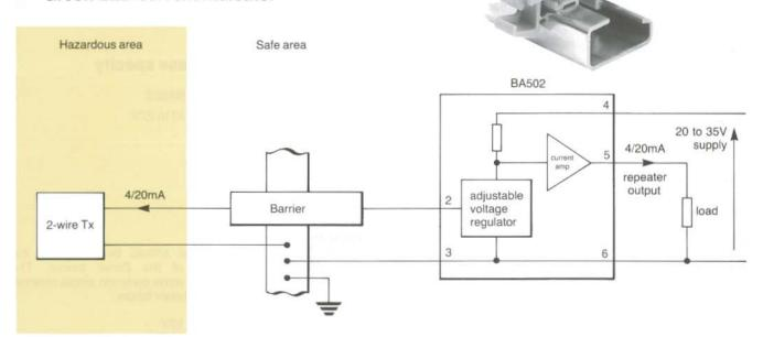
The BA502 current repeater provides Zener barrier protected loops with greater transmitter and load voltage, and allows higher supply voltages to be used without blowing expensive barrier fuses. In addition, the BA502 eliminates the need for a return Zener barrier in systems operating from a common power supply, thus only one low cost single channel barrier is required for each loop.
