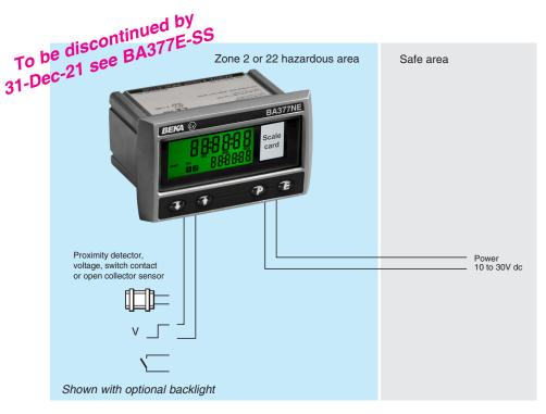
The BA377NE timer or clock has a rugged stainless steel enclosure allowing it to be safely installed in an Ex n or Ex to panel enclosure located in Zones 2 or 22 without the need for Zener barriers or galvanic isolators. The instrument is easy to use and can be configured on-site to operate with sensors having a wide variety of outputs. A slide-in scale card simplifies identification.
