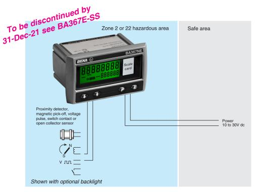
The BA367NE has a rugged stainless steel enclosure with Ex nA and Ex to certification allowing it to be safely installed in an Ex n or Ex to panel enclosure located in Zones 2 and 22, without the need for Zener barriers or galvanic isolators. The counter is easy to use and can be configured on-site to operate with a wide variety of sensors. A slide-in scale card simplifies identification.
