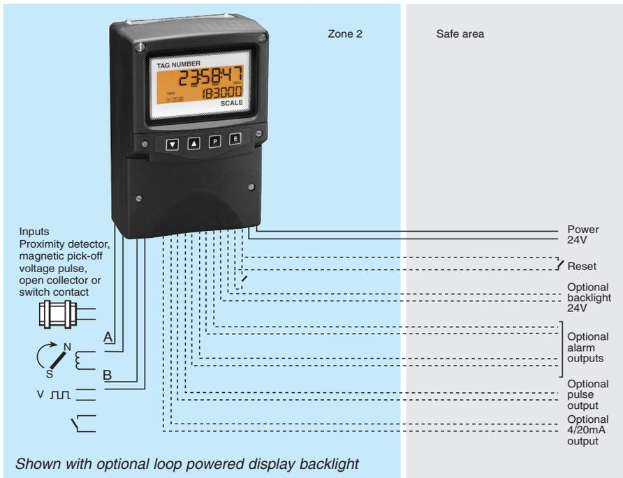
The **BA364ND** is a Type nL certified multi-function instrument which may be programmed to perform a host of counting and timing functions. Easy to use menus allow the instrument to be configured as a counter, timer, tachometer or as a clock. Both of the inputs will operate from 2-wire proximity detectors, switch contacts, magnetic pick-offs, open collectors or voltage pulses. Optional alarm/control outputs further extend the many applications.
