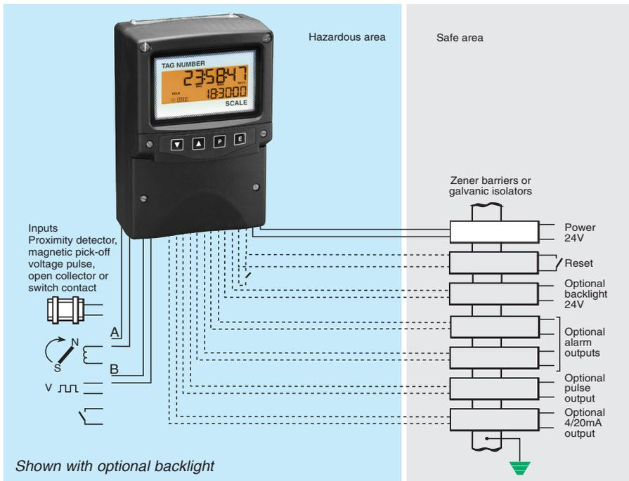
The **BA364D** is an intrinsically safe multi-function instrument which may be programmed to perform a host of counting and timing functions. Easy to use menus allow the instrument to be configured as a counter, timer, tachometer or as a clock. Both of the inputs will operate from 2-wire proximity detectors, switch contacts, magnetic pick-offs, open collectors or voltage pulses. Optional alarm/control outputs further extend the many applications.
