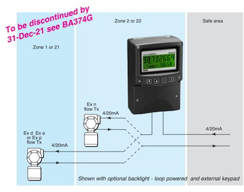
The BA354NE loop powered 4/20mA rate totaliser is a third generation field mounting instrument that is electrically and mechanically compatible with the earlier BA354ND, but it has a larger display, extended operating temperature and additional features such as a lineariser and bi-directional flow capabilities. Like its predecessor the BA354NE is housed in a robust IP66 GRP enclosure with a separate terminal compartment.
