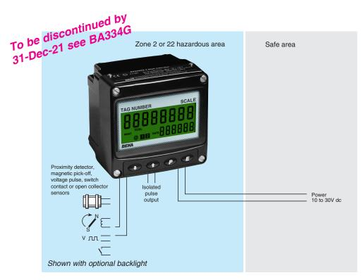
The BA334NG is a third generation field mounting rate totaliser housed in a compact IP66 GRP enclosure. The totaliser is easy to use and can be configured on-site to operate with flowmeters having a magnetic pick-off, switch contact, proximity detector, open collector or a voltage pulse output. International Ex nA and Ex tc certification permits worldwide installation in Zones 2 or 22 without Zener barriers or galvanic isolators which significantly reduces installation cost.
