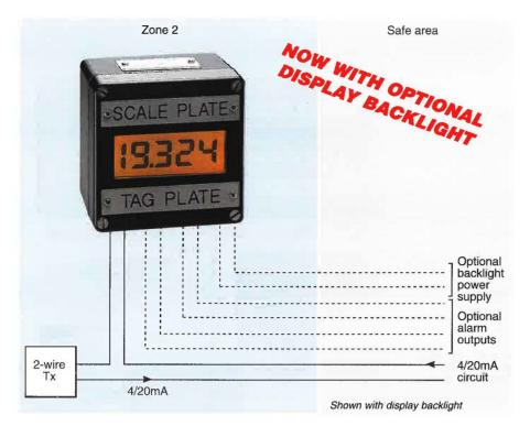
The BA324NC is a Type N field mounting indicator which displays the current flowing in a 4/20mA loop in meaningful engineering units. BA324NC has a 20mm high, easy to read liquid crystal display, and is housed in a robust IP66 enclosure. Modular accessories enable only the required features to be incorporated thus while reducina cost retaining interchangeability between instruments.
