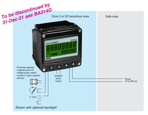
The BA314NG is a third generation field mounting tachometer housed in a compact IP66 GRP enclosure. The tachometer is easy to use and can be configured on-site to operate with a magnetic pick-off, switch contact, proximity detector or open collector sensor. International Ex nA and Ex to certification permits worldwide installation in Zones 2 or 22 without Zener barriers or galvanic isolators which significantly reduces installation costs.
