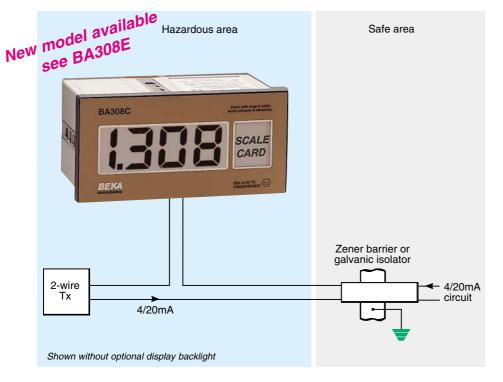
The BA308C is an intrinsically safe panel mounting indicator which displays the current flowing in a 4/20mA process loop in meaningful engineering units. The instrument is loop powered but only introduces a 1V drop allowing it to be installed in series with almost any 4/20mA loop.
