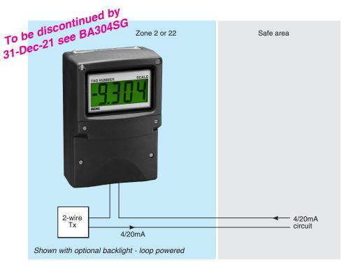
The BA304NE loop powered 4/20mA indicator is a fourth generation field mounting instrument that is mechanically compatible and electrically similar to the earlier BA304ND. It has a much larger full 4 digit display and guaranteed performance between -40 and 70°C. Like it's predecessor, the BA304NE is housed in a robust IP66 enclosure with a separate terminal compartment.
