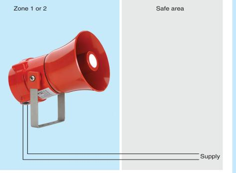
The BExS110D solid state electronic sounder produces a loud audible warning signal within a hazardous area. To avoid confusion between alarm signals, the sounder can be conditioned by internal switches to generate any one of thirty two unique alarm sounds. Maximum continuous output is 117dB(A) at 1m. **ATEX flameproof certification** allows all models to be installed in Zone 1 or 2, and to be used with gases in groups IIA, IIB and IIC.
