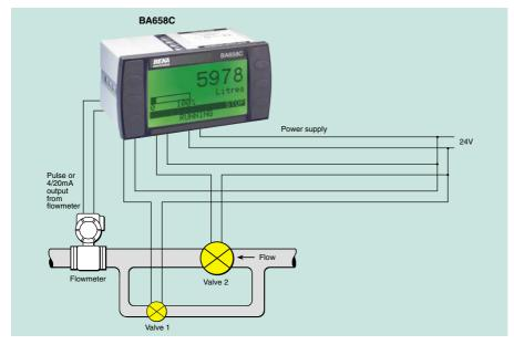
The BA658C is a second-generation, general-purpose flow batch controller that supersedes the successful BA550P and BA550C. This controller is ideal for accurately dispensing liquids, solids or components and despite its sophisticated control functions, it remains very easy to use and configure.
