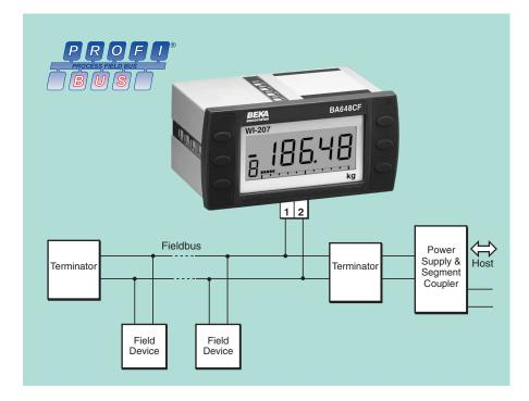
The BA648CF-P PROFIBUS Indicator is a general purpose instrument that can display up to eight fieldbus process variables. A numeric annunciator on the left hand side of the screen shows which variable is being displayed. This version of the indicator supports PROFIBUS PA protocol; for FOUNDATION™ fieldbus systems an alternative version is available -please see BA648CF-FFOUNDATION™ fieldbus datasheet.
