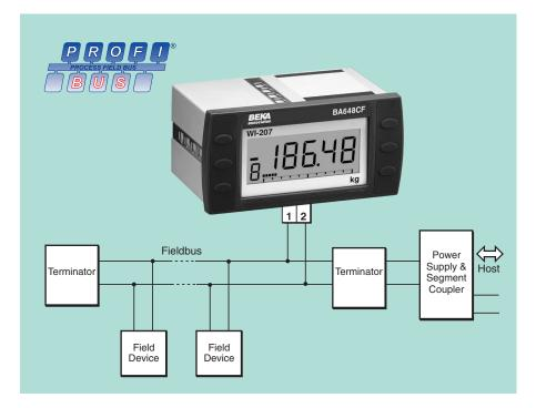
The BA648CF-P PROFIBUS Indicator is a general purpose instrument that can display up to eight fieldbus process variables. A numeric annunciator on the left hand side of the screen shows which variable is being displayed. This version of the indicator supports PROFIBUS PA protocol; for FOUNDATION™ fieldbus systems an alternative version is available -please see BA648CF-FFOUNDATION™ fieldbus datasheet.
