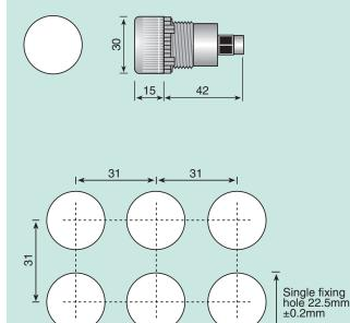
Fixing centres for maximum packing density. Special tool may be required to tighten fixing nuts when minimum spacing is used.
