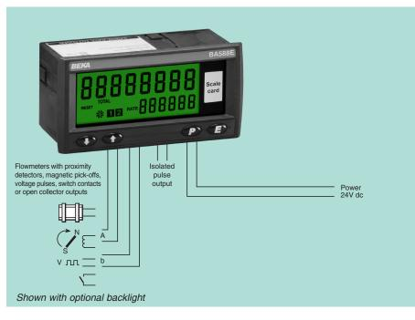
**The BA588E** is a two input general purpose rate totaliser that can simultaneously display the total flow and the rate of flow of either flowmeter, or the sum or difference of the two inputs. Rate and total displays may have the same or different engineering units. The BA588E is easy to use and each input can be independently configured on-site to operate with a flowmeter having various pulse outputs. A slide-in scale card simplifies identification.
