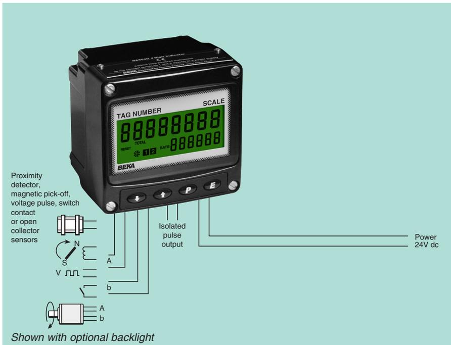
The **BA564G** is a third generation, field mounting two input counter housed in a compact IP66 GRP enclosure. The counter is easy to use and each input can be individually configured on-site to operate with sensors having a magnetic pick-off, switch contact, proximity detector, open collector or a voltage pulse output. Alternatively, the two counter inputs can be used for decoding the output from a quadrature position encoder.
