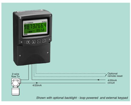
The BA554E loop powered 4/20mA rate totaliser is a third generation, general purpose, field mounting instrument that is electrically and mechanically compatible with the earlier BA554D, but it has a larger display, extended operating temperature and additional features such as a lineariser and bi-directional flow capabilities. Like its predecessor the BA554E is housed in a robust IP66 GRP enclosure with a separate terminal compartment
