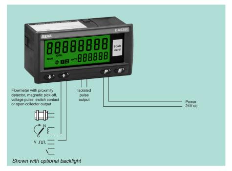
The BA538E is a third generation general purpose rate totaliser that is compatible with the earlier BA538C, but has a much larger display, a lineariser and an isolated synchronous pulse output. The totaliser is easy to use and can be configured on-site to operate with flowmeters having a magnetic pick-off, switch contact, proximity detector, open collector or a voltage pulse output. A slide-in scale card shows the units of measurement and simplifies identification.
