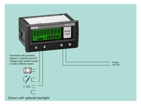
The BA537E is a third generation general purpose rate totaliser that has similar functions as the BA538E, but is housed in a smaller 96 x 48mm DIN enclosure. The totaliser is easy to use and can be configured on-site to operate with flowmeters having a magnetic pick-off, switch contact, proximity detector, open collector or a voltage pulse output. A slide-in scale card shows the units of measurement and simplifies identification.
