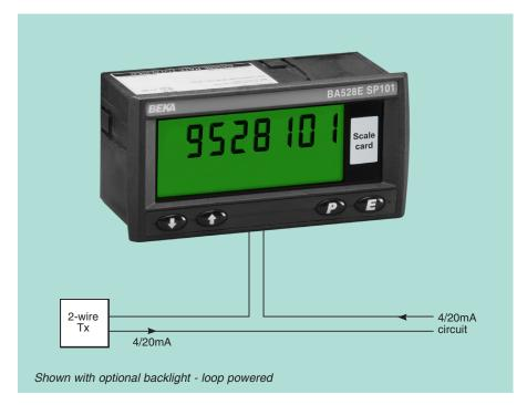
The 7 digit BA528E SP101 loop powered 4/20mA indicator is a special version of the BA528E indicator, featuring two additional least significant digits, which may be configured to be active digits, or dummy trailing zeros.
