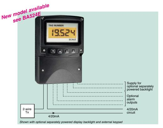
The new BA524D is a third generation, general purpose field mounting indicator housed in a robust IP66 GRP enclosure incorporating a separate terminal compartment and dedicated access to the instrument controls. Retaining all the features of the popular BA524C, this new indicator provides improved display visibility, plus simplified installation, calibration and routine inspection facilities.
