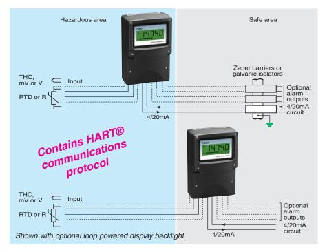
The BA474D is a second generation, intrinsically safe, loop powered indicating temperature transmitter. It provides an accurate local digital temperature display, plus a 4/20mA output, which may be scaled to represent any temperature range. The BA474D incorporates HART® digital communication, associated apparatus certification and a robust GRP enclosure with a separate terminal compartment.
