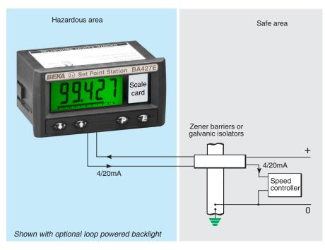
**The BA427E** is an intrinsically safe panel mounting set point station that enables the current flowing in a 4/20mA loop to be manually adjusted via the front panel push buttons from within the hazardous area. It is a second generation instrument that is mechanically and electrically compatible with the earlier BA405C, but has more display digits plus additional functions.
