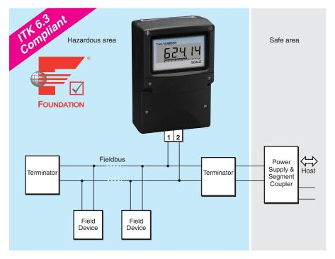
The BA414DF-F Fieldbus Indicator is a cost-effective intrinsically safe field mounting instrument that displays a single fieldbus process variable in a hazardous area. Housed in a robust IP66 GRP enclosure, the instrument has a large, high contrast five digit display, plus a horizontal bargraph. The BA414DF-F indicator uses the same technology and compliments the well established BEKA eight variable fieldbus displays that are now in worldwide use.
