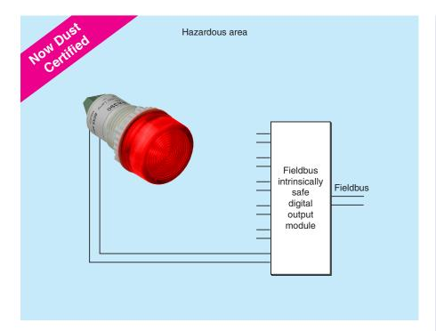
BA390S low current panel lamps provide reliable, cost effective visual status indication in all gas and dust hazardous areas. Each BA390S lamp produces a uniform output with just a few milliamps of input current and has a typical life greater than ten years.
