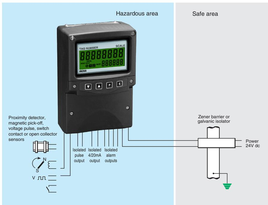
The **BA384E** is a two input, field mounting, intrinsically safe rate totaliser that can simultaneously display the total flow and rate of flow of either flowmeter, or the sum or difference of the two. The BA384E is easy to use and each input can be individually configured on-site to operate with a flowmeter having a variety of pulse outputs. International intrinsic safety certification permits worldwide installation.
