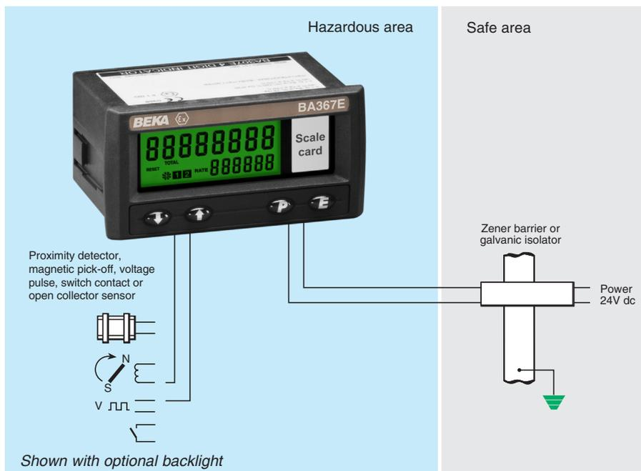
The **BA367E** is a one input intrinsically safe counter with one input that has similar functions as the two input BA368E, but is housed in a smaller 96 x 48mm DIN enclosure. The counter is easy to use and can be configured on-site to operate with magnetic pick-off, switch contact, proximity detector, open collector or a voltage pulse sensor. A slide-in scale card simplifies identification and international intrinsic safety certification permits worldwide installation.
