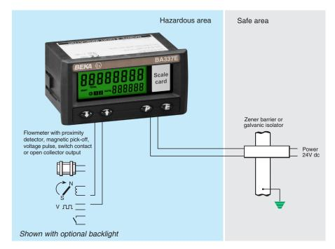
The BA337E is a third generation intrinsically safe rate totaliser that has similar functions as the BA338E, but is housed in a smaller 96 x 48mm DIN enclosure. The totaliser is easy to use and can be configured on-site to operate with flowmeters having a magnetic pick-off, switch contact, proximity detector, open collector or a voltage pulse output. A slide-in scale card simplifies identification and international intrinsic safety certification permits worldwide installation.
