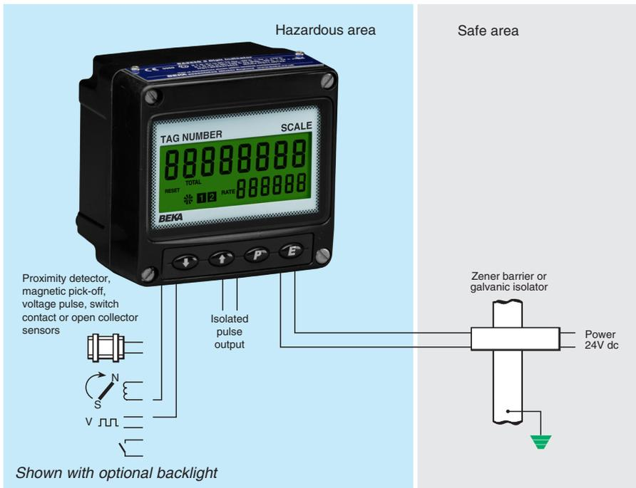
The **BA334G** is a third generation intrinsically safe field mounting rate totaliser housed in a compact IP66 GRP enclosure. The totaliser is easy to use and can be configured on-site to operate with flowmeters having a magnetic pick-off, switch contact, proximity detector, open collector or a voltage pulse output. International intrinsic safety certification permits worldwide installation.
