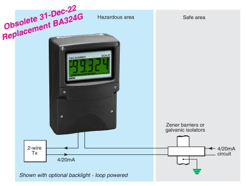
The BA324E loop powered 4/20mA indicator is a fourth generation field mounting instrument that is electrically and mechanically compatible with the earlier BA324D. It has a much larger full 5 digit display and guaranteed performance between -40 and 70°C. Like it's predecessor, the BA324E is housed in a robust IP66 enclosure with a separate terminal compartment.
