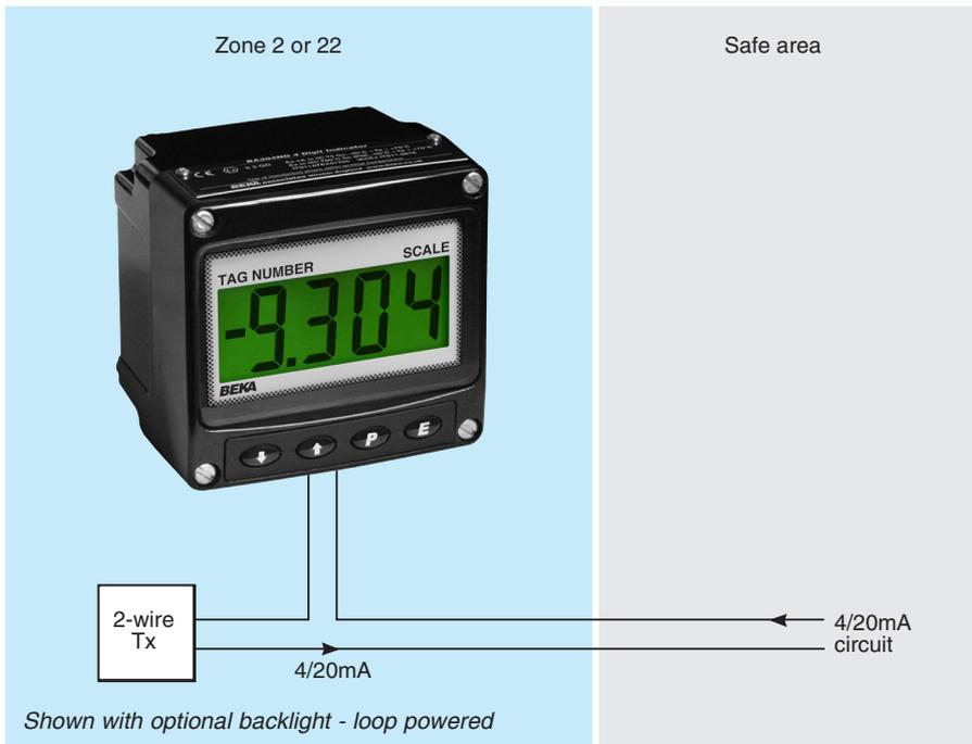
The **BA304NG loop powered 4/20mA indicator** is a new field mounting instrument that supersedes the well established BA304NC. It is electrically and mechanically compatible with the earlier model but has a much larger full 4 digit display, dust certification and guaranteed performance between -40 and +70°C. Like its predecessor, the BA304NG is housed in a robust IP66 enclosure which may be surface or pipe mounting.
