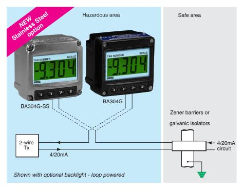
The BA304G loop powered 4/20mA indicator is an intrinsically safe field mounting instrument with a large 4 digit display housed in a robust IP66 GRP or stainless steel enclosure.
