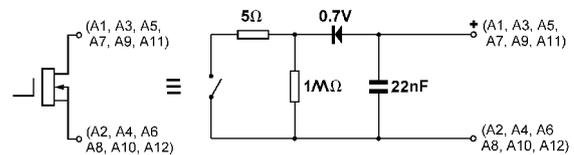
Fig 4 Equivalent circuit of each switch output
