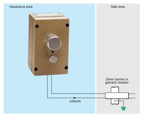
The BA404B manual set point station enables the current flowing in a 4/20mA loop to be adjusted from the process area. The instrument is loop powered, and has been certified intrinsically safe allowing installation within a hazardous area.
