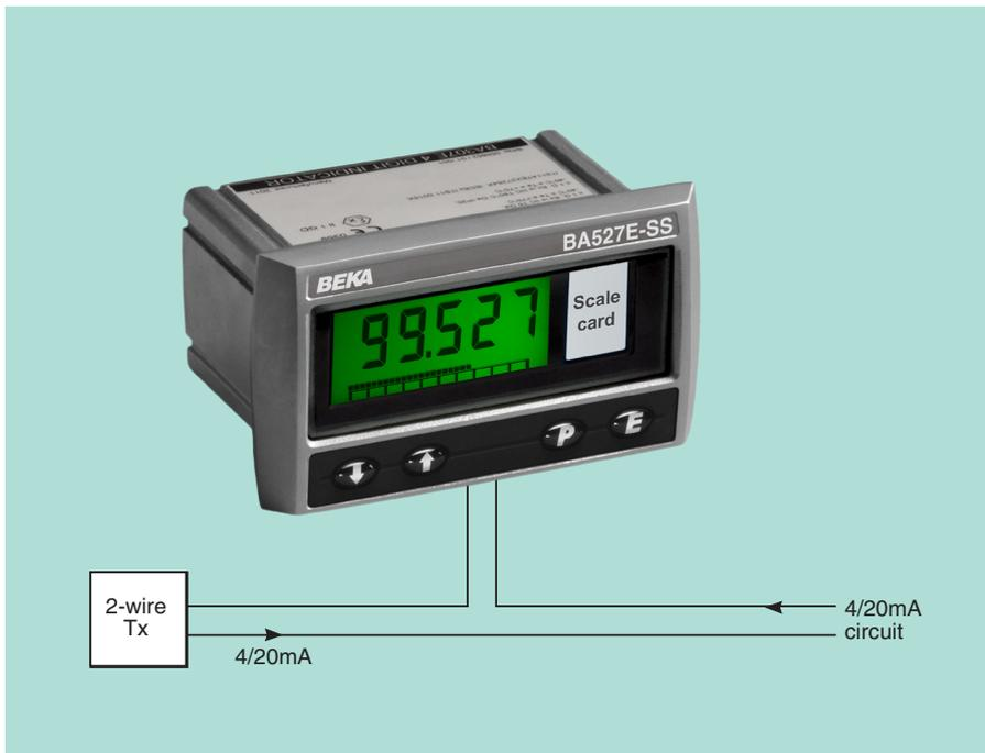
The **BA527E-SS** rugged general purpose, panel mounting 4/20mA loop powered Indicator, has a stainless steel housing allowing it to be safely installed in harsh industrial and marine environments, or where the front of the instrument is likely to be impacted. Incorporating a full 5 digit display plus a 31 segment bargraph with guaranteed performance between -40 and 70°C, the indicator can be calibrated to show the 4/20mA input current in almost any engineering units.
