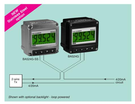
The BA524G is a general purpose, loop powered 4/20mA field mounting indicator, with a large five digit display and a bargraph housed in a robust IP66 GRP or stainless steel enclosure.
