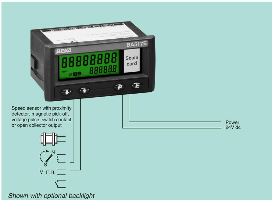
The BA517E is a third generation general purpose tachometer that has similar functions as the BA518E, but is housed in a smaller 96 x 48mm DIN enclosure. The tachometer is easy to use and can be configured on-site to operate with a magnetic pick-off, switch contact, proximity detector, open collector or voltage pulse sensor. A slide-in scale card can be supplied printed with units of measurement, or can easily be marked on-site.
