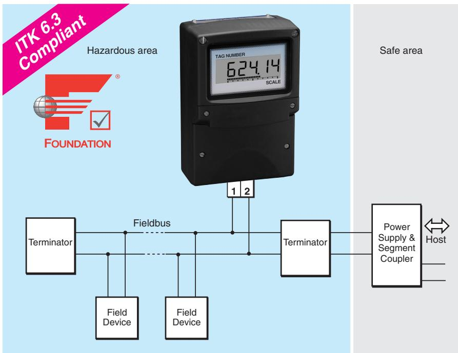
**The BA414DF-F Fieldbus Indicator** is a cost-effective intrinsically safe field mounting instrument that displays a single fieldbus process variable in a hazardous area. Housed in a robust IP66 GRP enclosure, the instrument has a large, high contrast five digit display, plus a horizontal bargraph. The BA414DF-F indicator uses the same technology and complements the well established BEKA eight variable fieldbus displays that are now in worldwide use.
